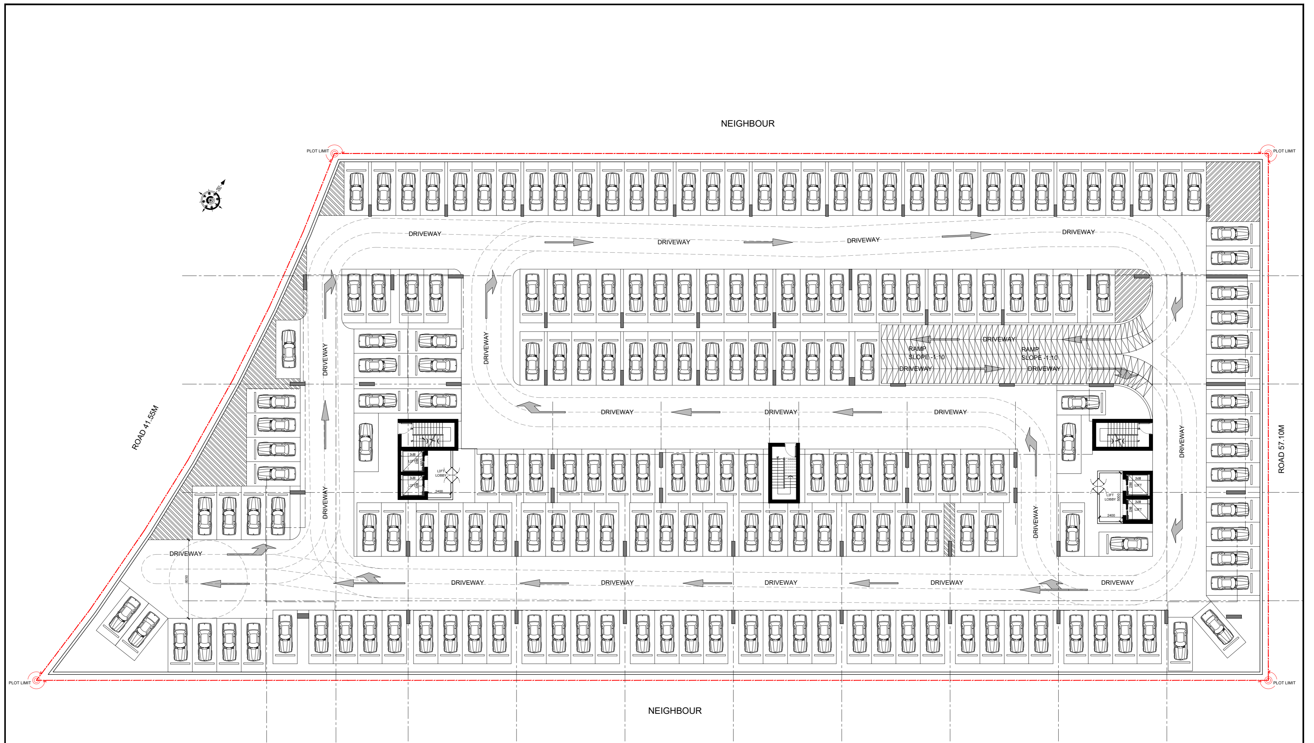
BASEMENT FLOOR PLAN 1 TOTAL NO.OF PARKING - 192 NO.S
